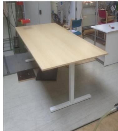
**Test method** Determination of strength, durability and safety of non-domestic table presented in the standard EN 15372: 2008 Furniture – Strength, durability and safety – Requirements for non-domestic tables. Selected type on usage was level 2.
