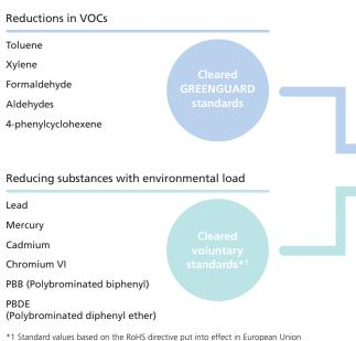
\*1 Standard values based on the RoHS directive put into effect in European Union member states in July 2006 to restrict the use of hazardous substances in electronic and electrical equipment. These standard values contain exemptions set in the RoHS directive.
